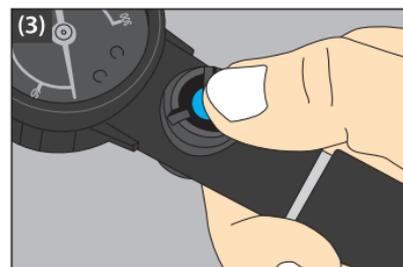
Micro adjust the pressure by pressing the air-bleeder
