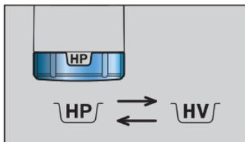
Switch between High Pressure (HP) and High Volume (HV)
