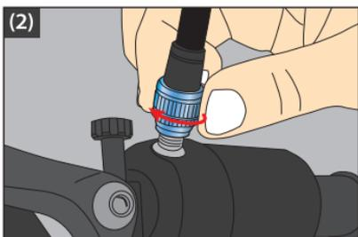
Screw the pump head in the valve until tightened then inflate
